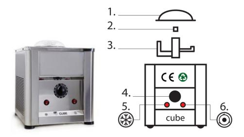
MINIGEL750 is Ideal for families & small restaurants, prepares up to 1 1/2 quarts (1.5 liters) of homemade gelato, ice cream, sorbet and frozen yogurt per hour. All MINIGEL are made with sustainable materials. Width: 11.8 in Height: 11.8 in Depth: 11.8 in Weight: 35.3 Refrigerant: R134a (70 grams) Power (HZ): 140W Voltage (W): 220V/50Hz Absorbed electricity (A): 1,5 Type of gas used: R134a Full gas capacity (G): 85
